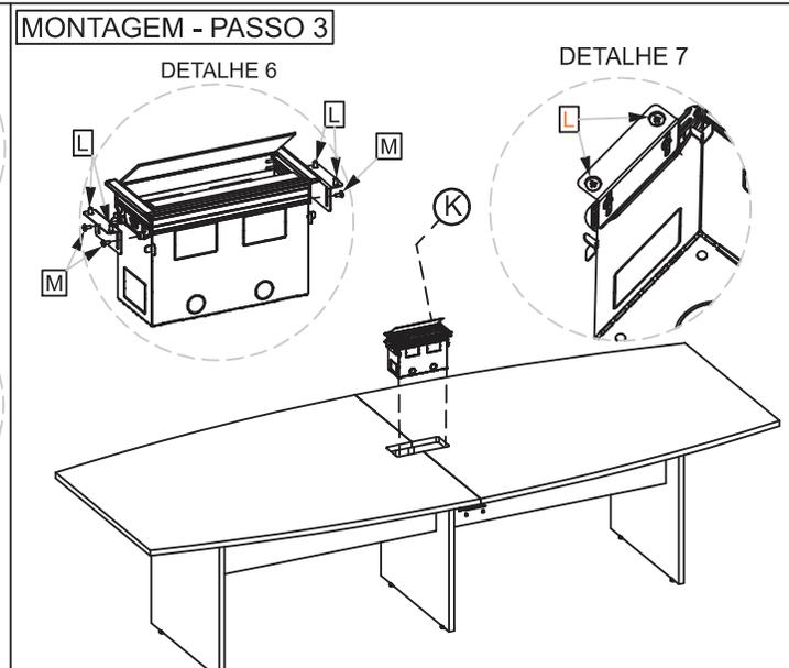
PARA FINALIZAR A MONTAGEM, ENCAIXE A CAIXA BASIC (K) NOS TAMPOS E FIXE OS SUPORTES LATERAIS NA CAIXA CONFORME O DETALHE 5, PARA QUE MESMA POSSA SER FIXADA NOS TAMPOS (1) CONFORME INDICA O DETALHE 7.
