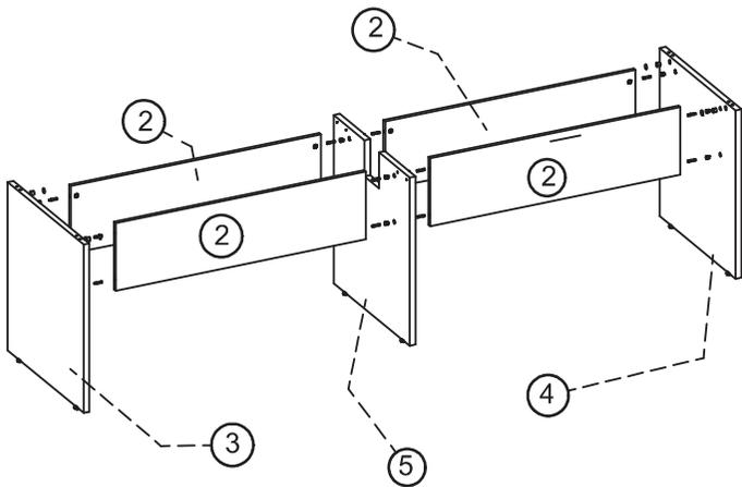
INICIE MONTANDO A ESTRUTURA: FIXE O PÉ PAINEL ESQUERDO (3), EM SEGUIDA FIXE O PAINEL CENTRAL (2), DEPOIS FIXE O PÉ CENTRAL (5), DEPOIS FIXAR O PAINEL CENTRAL (2) E POR ULTIMO FIXE O PÉ LATERAL DIREITO (4).
